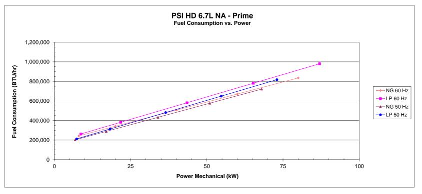
Technical data based on ISO 3046-1 standards of 77°F (25°C), barometric pressure of 14.5Psia (100kPa) and 30% relative humidity. Production tolerances in engines and installed components can account for power variations of ± 5%.
